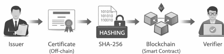
Figure 2. Architecture of the proposed blockchain-based competency certificate verification system
